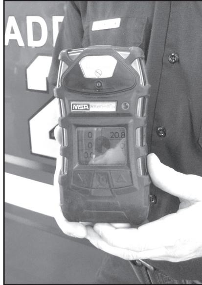
Air quality device detects gases that explode or are deadly to breathe.
